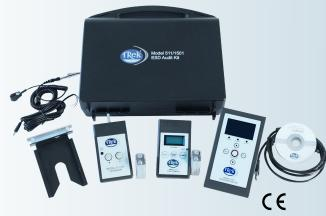
Trek's Model 511/1501 Electrostatic Discharge (ESD) Audit Kit includes the Model 511 Ionizer Kit (Model 511 Electrostatic Field Meter with charger and charge plate) and Model 1501 Surface Resistance Meter in a compact carrying case. Most items can be ordered individually.
